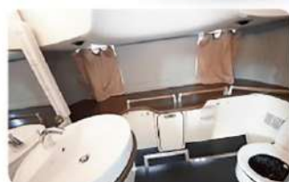
There is a powder room with a western-style toilet having noise-masking function.
